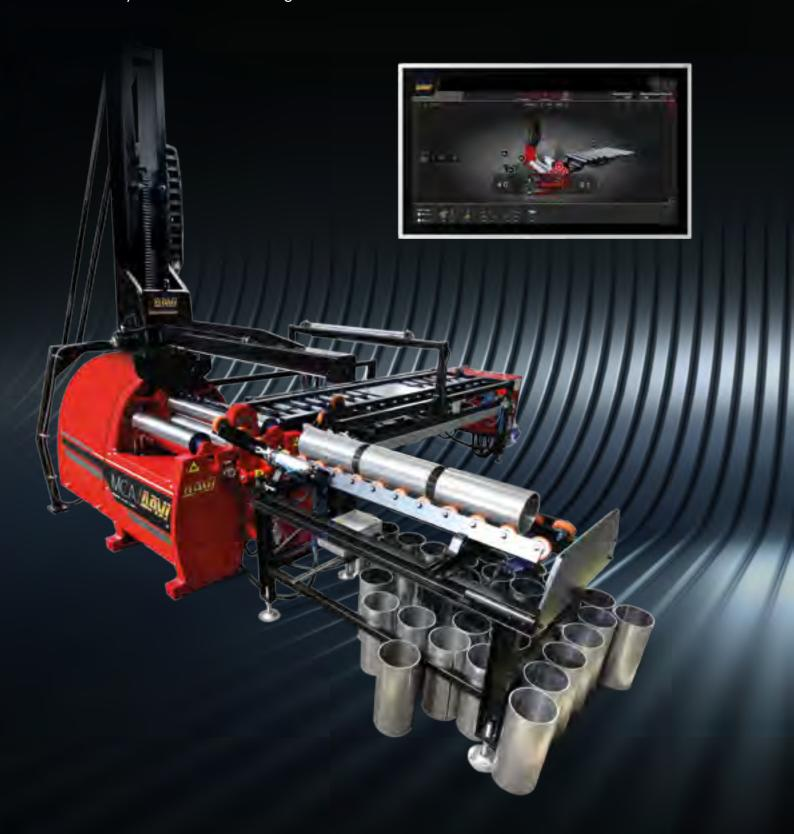
Davi Control System, tailored for the highest possible level of automation on the Market, features the possibility of automatically generating a full program importing the workpiece CAD file, recalling workpiece data from local network database through a barcode reader-based system and making use of offline Capacity and Spring-back Performance Test.
