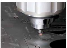
Flash Cut strategies synchronize turning the laser ON / OFF with axis movement to increase throughput.
