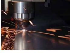
Pierce Detection senses when the pierce breaks through the material compared to a programmed pierce that would include added time to account for variations in the process.
