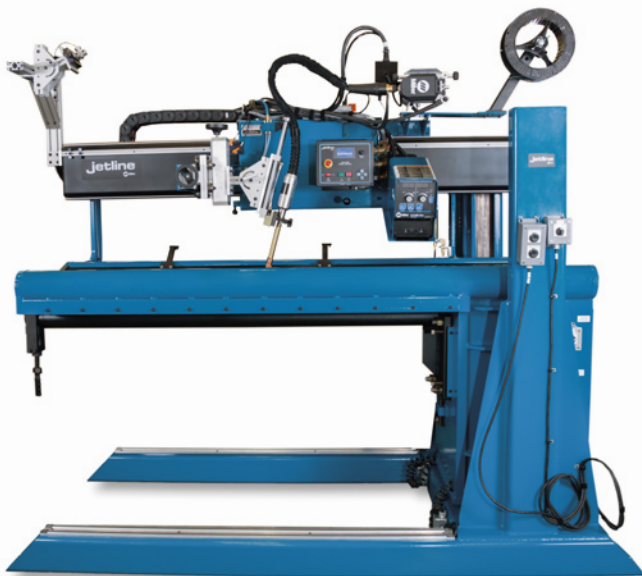
LWH elevating-style seam welder shown in lowered position.
