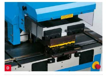
**Radiusing Unit** Various pre-sets for instant corner radiusing (3-15 mm radii) in material up to 5 mm thick.
