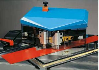
**Extended Cutting Length** Our notchers cut repeatedly in a straight line, infinitely extending the cutting length, while increasing notching capacity to 400 x 400 mm.
