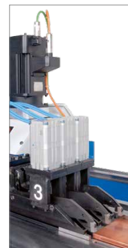
1-3 exchangeable clamps are used depending on the width of the bar
