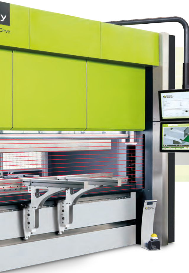
Integrated safety light guard
