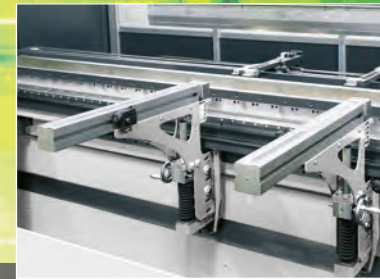
Moveable support arms adjustable in height
